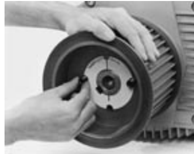
TIGHTEN SCREWS FINGER TIGHT
