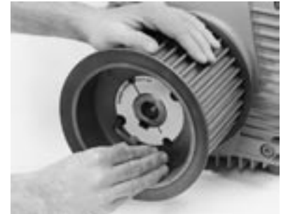
TIGHTEN SCREWS ALTERNATELY
