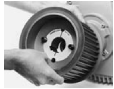
INSERT SCREWS AND LOCATE ON SHAFT
